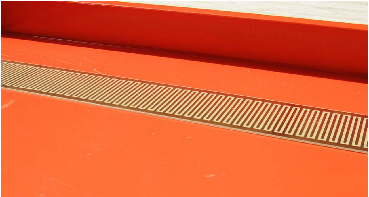
Application example: sensor circuit board KWS-3 in a collecting tray for condensate.
